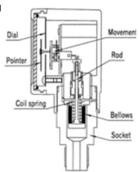
The movement has a special high-precision design and is made of parts with low coefficient of friction.
