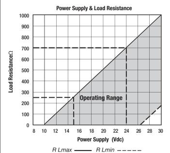
$\text{Maximum load resistance} \quad \frac{R_{L} max}{0.02(A)} \quad \frac{E\left(V\right) - 10(V)}{0.02(A)} \left(\Omega\right)$
