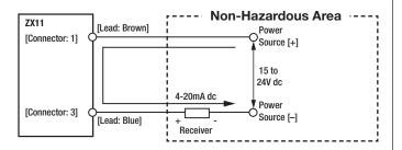
When connecting equipment that can generate surge from the same power supply, it is recommended that a voltage-dependent resistor (varistor) be connected to the pressure transmitter for protection. In addition, take the following precautions when wirina:
