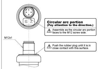
The "Z" on the rubber plug indicates the position of the potentiometer for zero adjustment, and the "S" indicates the position of the potentiometer for span adjustment.
