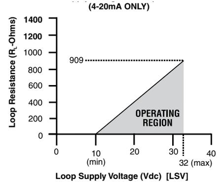
To determine minimum loop supply voltage:
